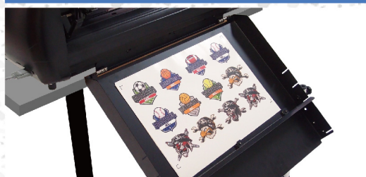
Media basket collects completed cutting sheets
