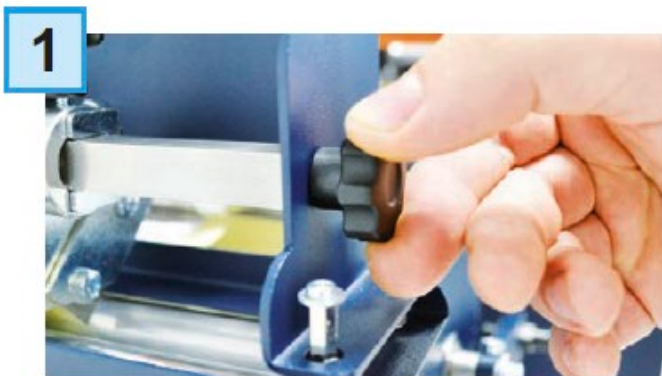
Remove the iron bar by unscrewing the black thumb screw.
