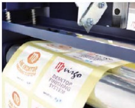
Pull the media through the aluminium rollers.
