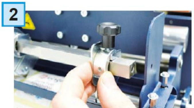
Slide the blade holder on or off. Replace the slide iron bar and rescrew the thumb screw
