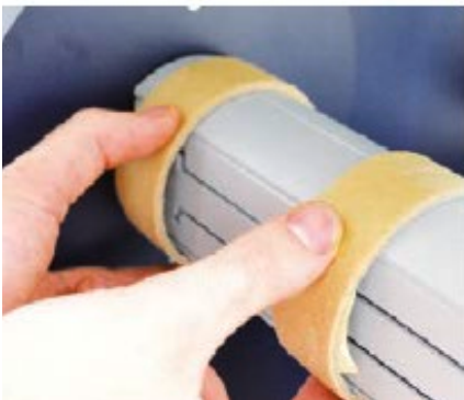
Load empty cardboard core(s) and tighten the core holder, then place the motorized core holder in position.
