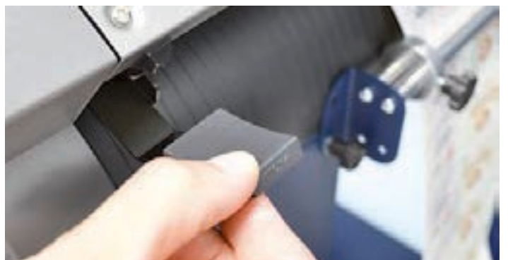
Put the lever, located in the rear of the plotter, in the down position.
