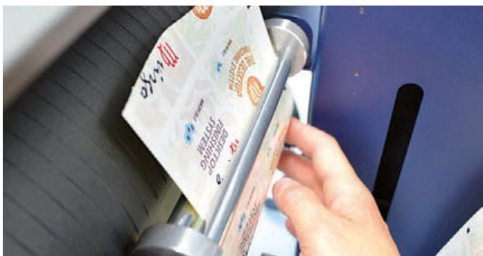
Pass it between the aluminium rollers. The guide can be adjusted to prevent the media from shifting.
