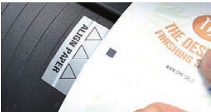
Pull the media through the plotter, keeping the media edge in contact with the alignment points.
