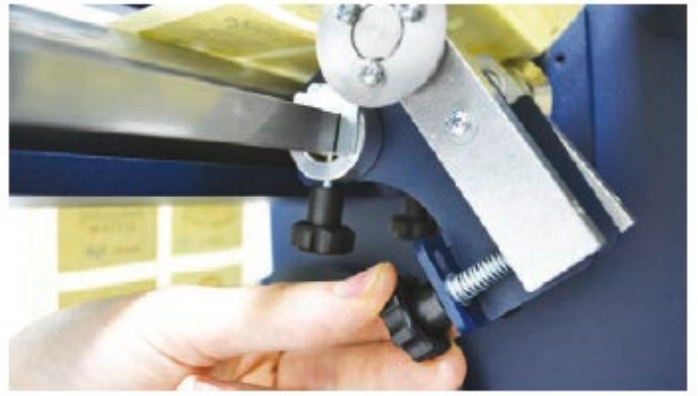
Use knob "B" to increase or decrease the force on the support. Clockwise: Increases the cutting force Counterclockwise: Decreases the cutting force
