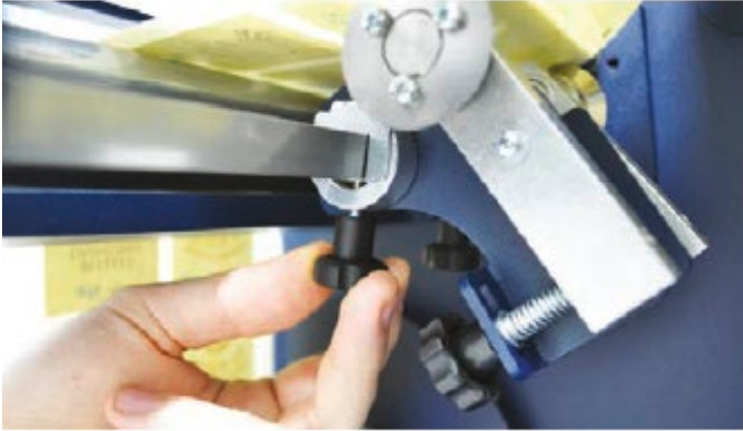
Tighten knob "A" to secure the position after choosing desired width .
