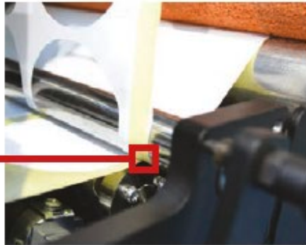
Relocate the o-rings to be over the waste matrix.
