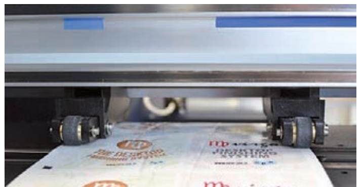
Set both pinch rollers at about 2 mm from the media edge.
